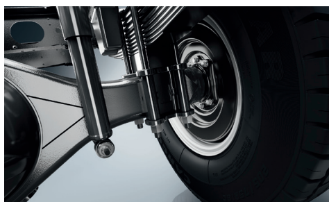
Rugged rear shock absorbers and multi-leaf suspension
