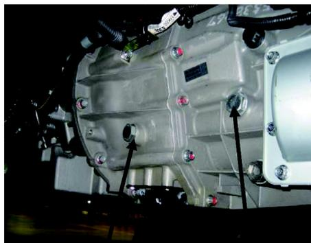
Automatic transmission fluid level plug
