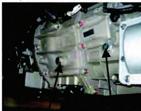
Automatic transmission fluid level plug Transmission gear oil fluid level plug
